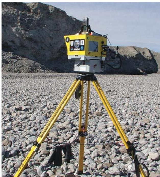
Figure 14. LIDAR setup.
